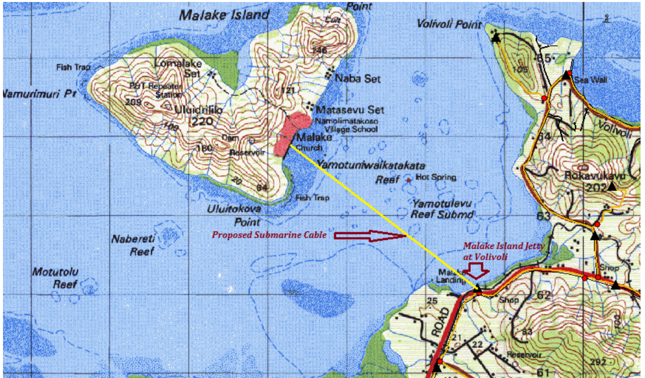
Figure 1: Submarine cable route from Malake Island Jetty (at Volivoli) to Malake Island.
