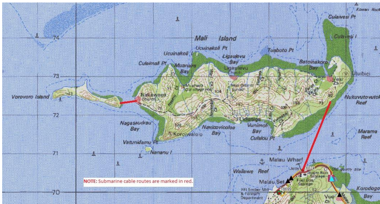
Figure 1: Submarine cable route from Malau Jetty to Mali Island and from Mali Island to Vorovoro Island.
