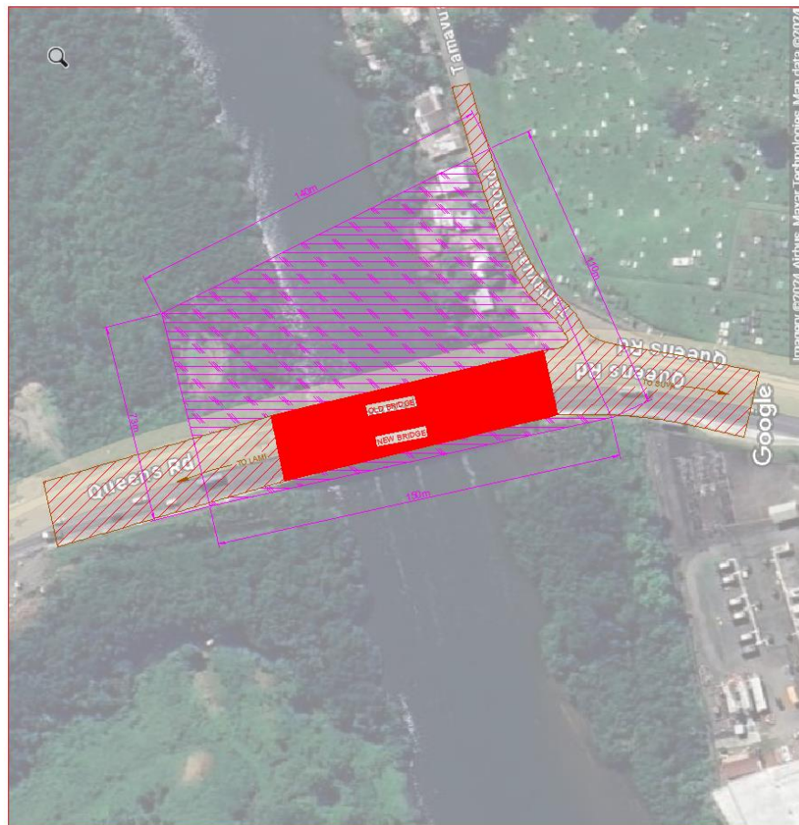
Figure 1: The area hatched on the Locality Map is area subjected to Topography Survey for Tamavua-i-wai.
