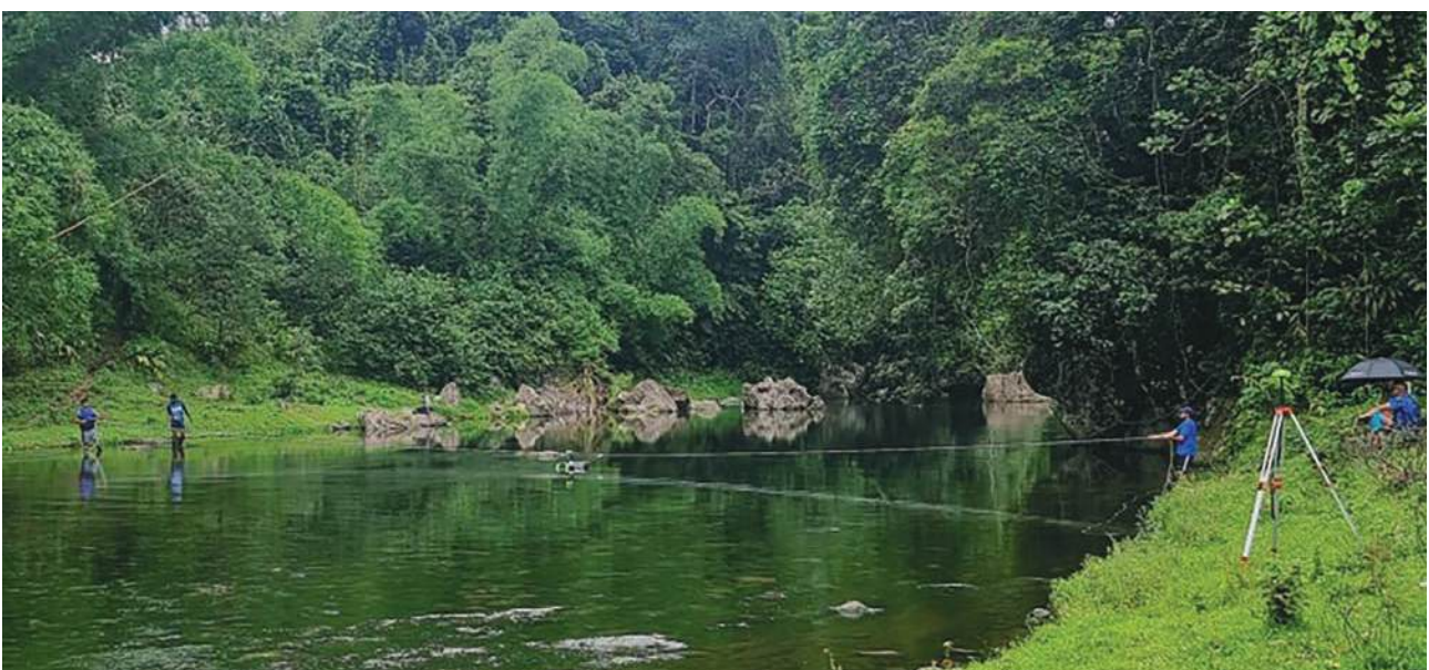
EFL Team carrying out survey works with Stantec undertaking River Flow Measurements at Wainikoroiluva River in interior Viti Levu
